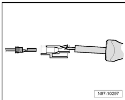
Terminal is ejected from the terminal housing.
