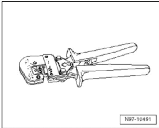
Crimp pliers VAS 1978/1A or crimp pliers (basic tool) VAS 1978/1-2 together with exchangeable head 0.35 - 2.5mm<sup>2</sup> VAS 1978/1-1 or exchangeable head 4.0 - 6.0mm<sup>2</sup> VAS 1978/2A from wiring harness repair kit is used to compress the crimp connections.
