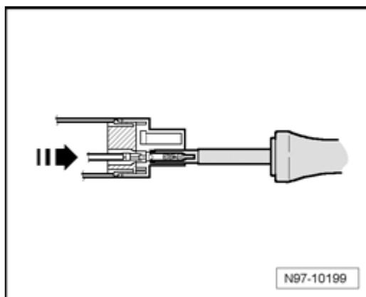
**Flat connector system with two retaining tabs:**
