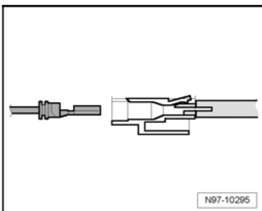
Terminal is ejected from the terminal housing.
