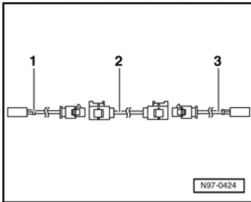
The entire length of the antenna wire consists of the length of the required adapter leads - **1** - and - **3** - as well as the connecting wire - **2** - .
