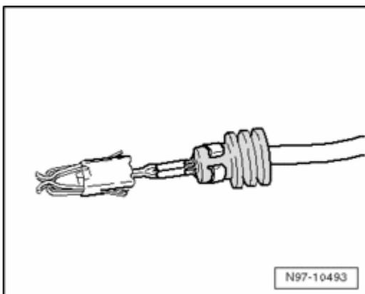
A correctly performed crimp is distinguished by a clean compression of wire and single wire seal in the terminal and has an impression on the rear side which identifies
