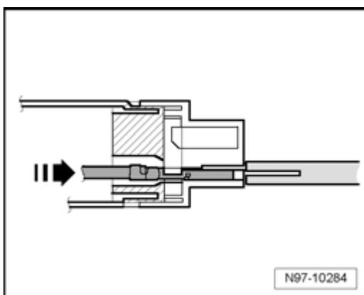
**Flat connector system with one retaining tab:**
