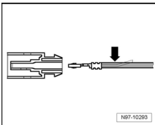
Assembly tools allow single wire seals to be slid into terminal housing up to stop without damage, this achieves a complete seal between single wire and terminal housing.
