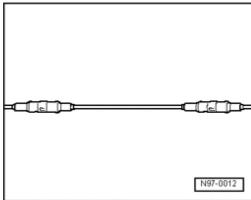
**Repair point with intermediate wire section**
