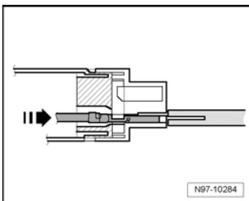
**Flat connector system with one retaining tab:**
