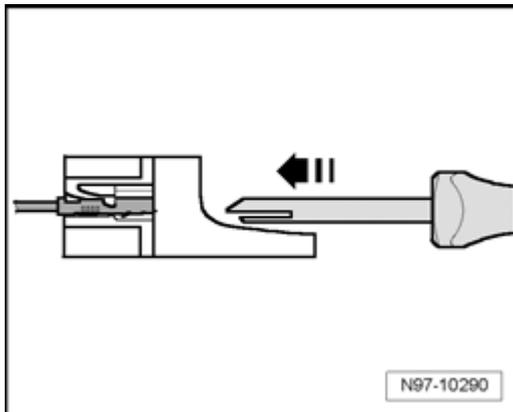
Various release tools are used to remove the different terminals from terminal housings without damage.
