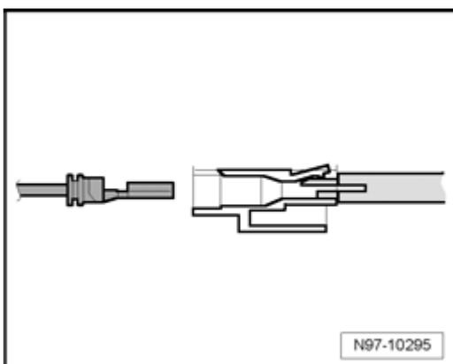
Terminal is ejected from the terminal housing.
