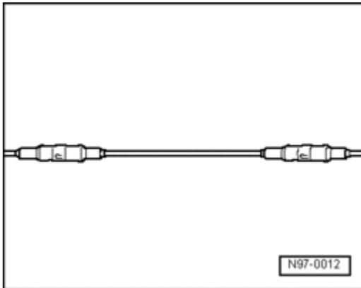
**Repair point with intermediate wire section**
