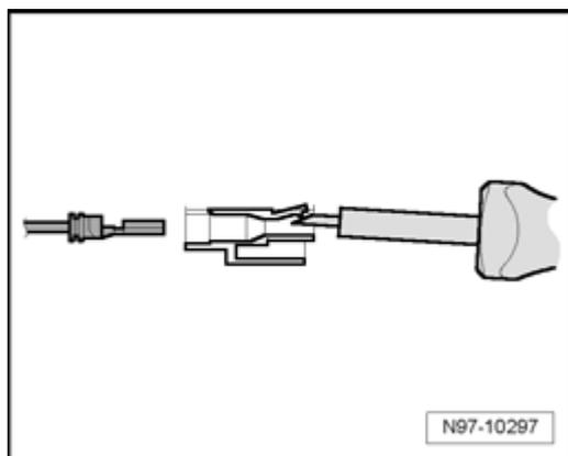
Terminal is ejected from the terminal housing.
