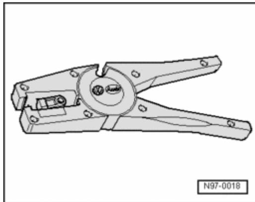
Wire Stripper VAS1978/3 is used for professional stripping and cutting of wires.
