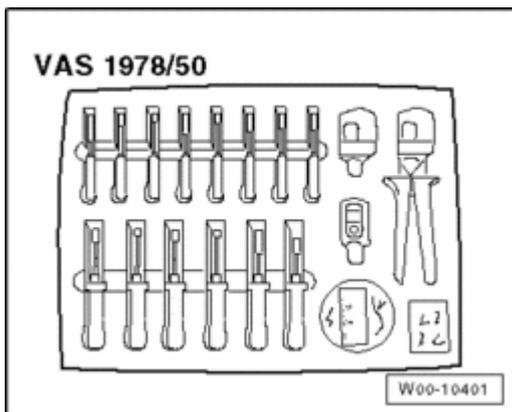
Upgrade kit VAS 1978/50 is required to bring the "old" Wiring Harness Repair Kit VAS1978 up to the new standard of Wiring Harness Repair Set VAS1978A . The upgrade kit contains 4 assembly- and 10 release tools as well as new crimp pliers for crimp connections with exchangeable heads for 0.35 mm - 2.5 mm VAS 1978/1-1 , 4.0 mm - 6.0 mm VAS 1978/2A and changeable head for JPT VAS 1978/9-1 . Furthermore it contains new
