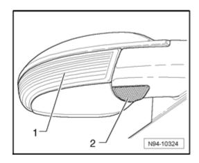
Turn signals and entry lights are integrated into the exterior mirror housings.
