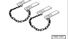
To prevent damage to edges of wings, cover lower areas of both adapters - 10 - 222 A /8- with woven adhesive tape -arrow-  $\Rightarrow$  Electronic Parts Catalogue (ETKA).
