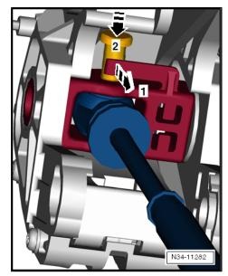
Secure the selector lever cable with a new securing plate to the cable bracket on the selector mechanism.
