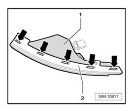
Using appropriate screwdriver, release retainers arrows - and remove clipped rub strip - 2 - from turn signal - 1 - .
