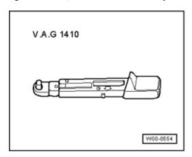
Torque wrench VAG 1410 (or 4 - 20 Nm equivalent)
