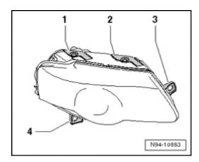
Should one or more headlamp securing lugs be damaged or broken, they can be replaced by installing the repair set. It is not necessary to replace the entire headlamp.
